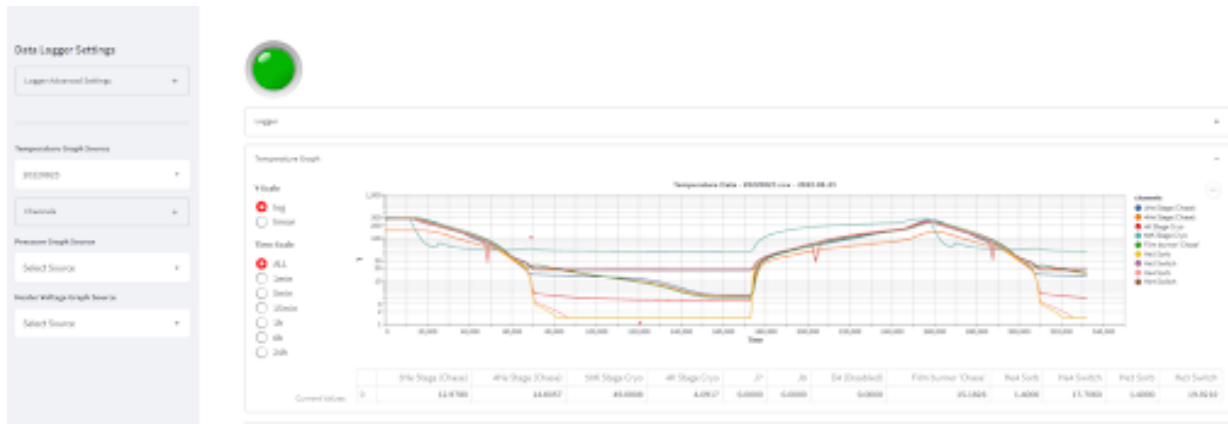
Figure 13: The Fridge Manager application developed for the 3He cryostat at SLAC. The GUI provides a user-friendly interface for monitoring and controlling the cryostat from any web browser. The graph shows the temperature of every stage of the cryostat over time, and can also display pressure and voltage data. The GUI allows the user to control data logger settings and remotely perform a fridge cycle.
