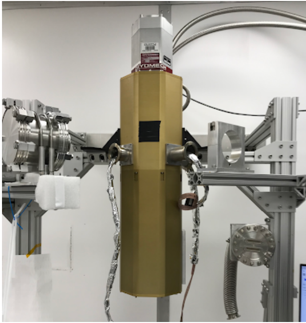
Figure 5: A 3He cryostat used for testing SPLENDOR readout electronics at SLAC national accelerator laboratory. Base temperature of \sim 300 mK.
